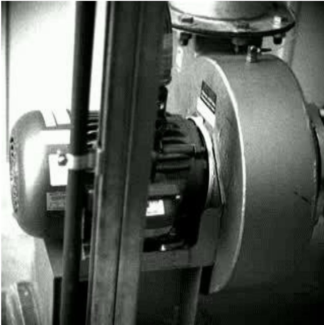
Figure 6: Frame of the MAV process applied to an industrial fan
