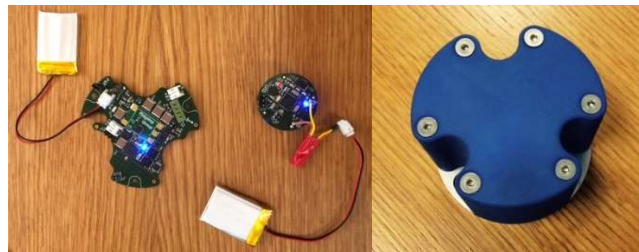
Figure 5. Boards with batteries and housing assembly
