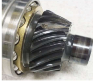
Figure 8. Failed gear – fractured tooth.
