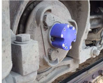
Figure 10: MEMS sensor mounted on a wheel hub
