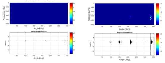
Figure 44. Angle-frequency spectrogram (left plot - healthy system, right plot - one day prior to a failure event).
