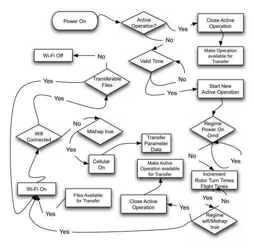
**Figure 1 Operation Finite State Machine**
