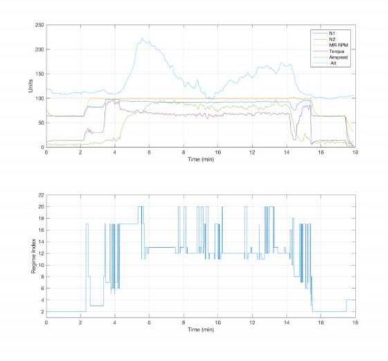
**Figure 3 Flight Parameters and Regime Index**
