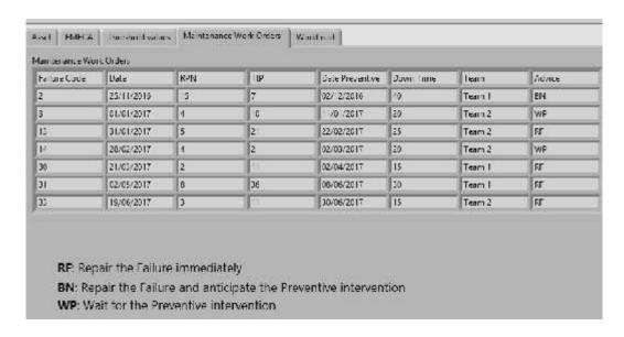
Figure 5: Maintenance Work Orders tab.
