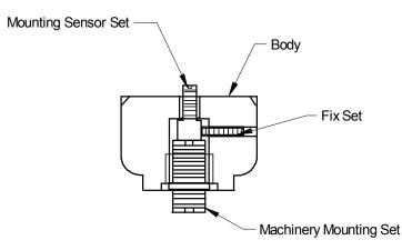
Figure 1. Structure diagram of universal sensor mount
