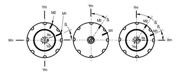
Figure 2. Illustration of the sensor mounting technology
