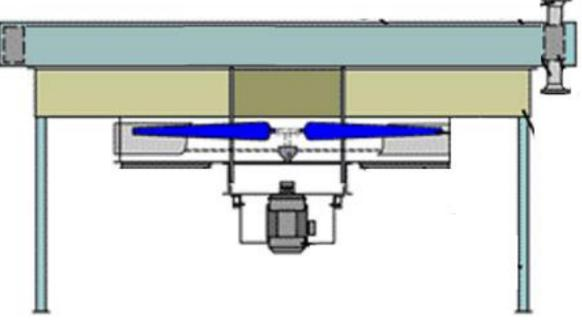
Fig 1: Fin Fan cooler with vertical mounted motor
