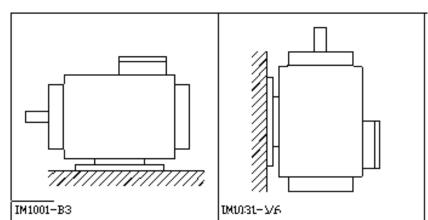
Fig 2: IEC 60034-7 based motor mounting (left – Horizonal mounting right – vertical mounting with plate)
