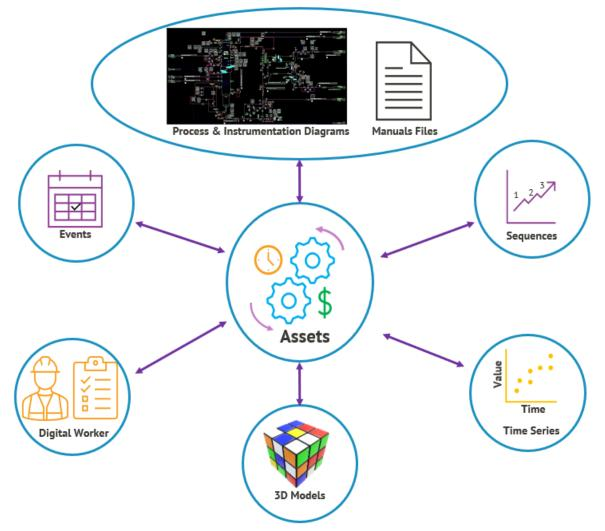
of start-up steps and checks. This is the start-up sequence. Motor current and vibration data from the pump is logged along with temperatures, pressures, and flows. These are time series data. The operations manuals provide limits on any of the data, sequence timing, etc. Our three (or two) dimensional models provide any visualization that is helpful to the operator or to management.
