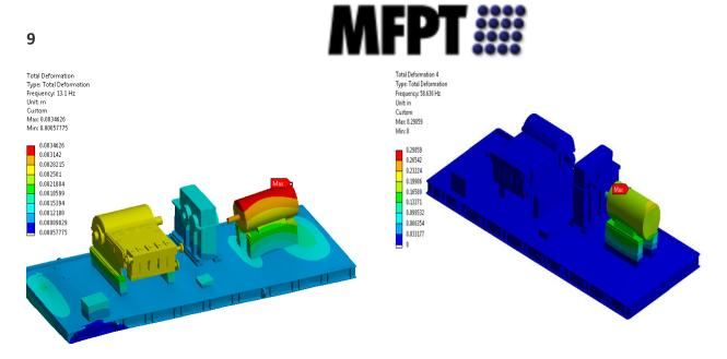
FE simulation results – As found (Left ABOVE) Motor pitching mode 13 Hz within 5% of calculated ODS and after grout (Right Above)
